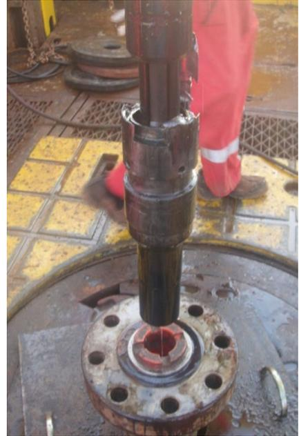
A Weatherford thru-tubing fishing services team retrieved a PX plug that was stuck downhole. This success eliminated the need for a costly recompletion operation and saved the operator 7 to 8 days of rig time.
