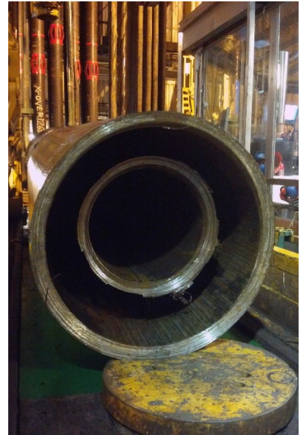
The M.O.S.T. Plus system cut cleanly through two strings of casing.
