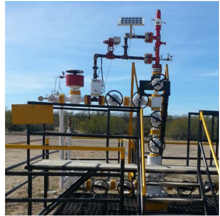
The Weatherford plunger-lift system with the WellPilot controller eliminated the need for daily chemical treatments and increased production rates to 15 BPD of condensate and 0.500 MMscfd.
