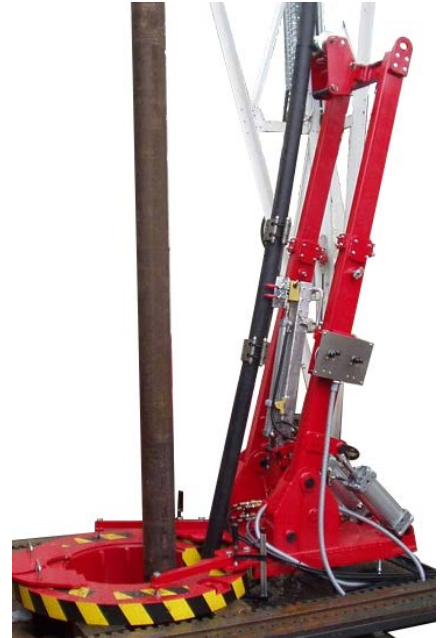
Weatherford AutoCLAMP safely and efficiently guiding the control lines.
