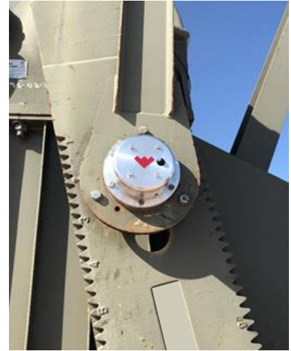
Foresite Sense equipment monitoring installs over the wrist-pin cap of surface-pumping units of all major brands.
