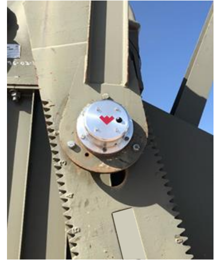
Foresite Sense installs over the wrist-pin cap of surface-pumping units of all major brands.
