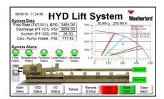
The Weatherford jet-lift automation system delivers trend analyses and real-time control over production parameters, including injection rates, pressures, and vibration management
