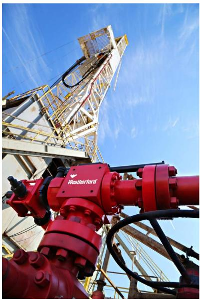
Cutline: The PressurePro control system fully integrates a rotating control device and electric choke for semi-automated wellbore pressure management.
