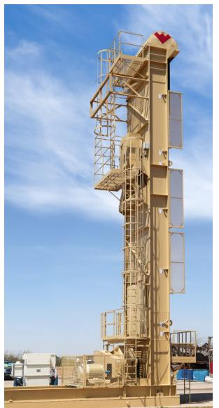
Cutline: The new Rotaflex long-stroke pumping unit leverages decades of field experience to provide operators with an easy-to-maintain, high-performance option for producing challenging wells.
