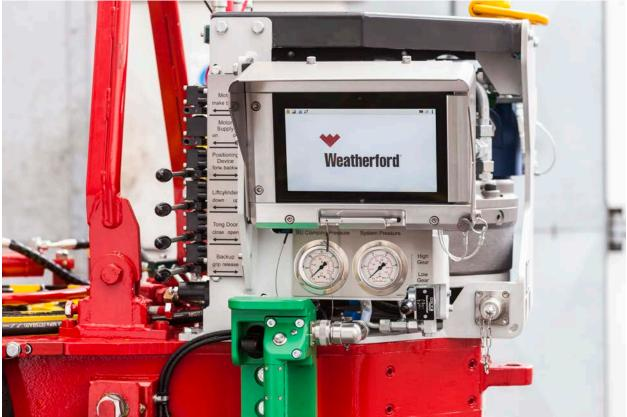
Cutline: The AutoTong system enhances the quality, consistency and efficiency of tubular connections by automatically making up pipe to the appropriate parameters.
