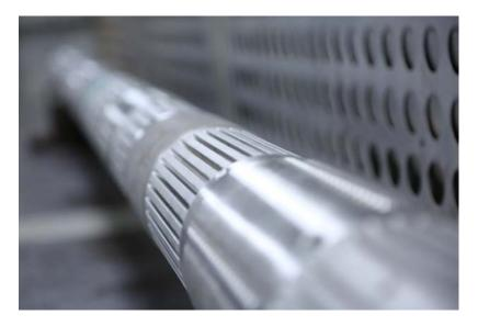
Cutline: HeatWave Extreme<sup>SM</sup> logging-while-drilling service reliably acquires gamma ray, resistivity, neutron porosity and density data at temperatures up to 200°C (392°F).
